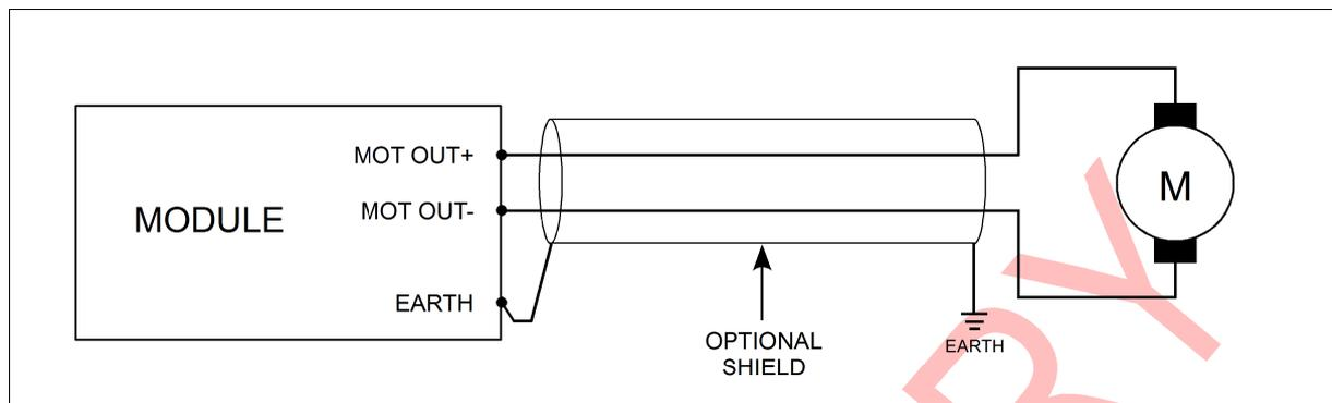
The wire cross-section should be suited to carry the current involved without excessive heating. Besides, the voltage drop along the cable should be kept low, especially in case of long distances; this might lead to the use of a larger copper cross-section.
