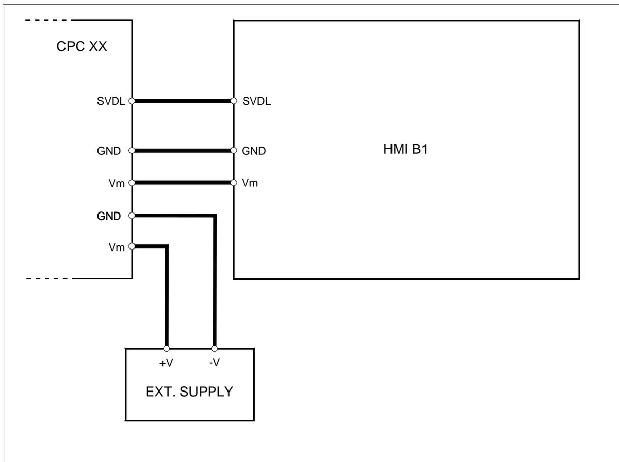
SDVL and power supply cables connecting CPC XX and HMI B1 must have the same length and should be bundled together.
