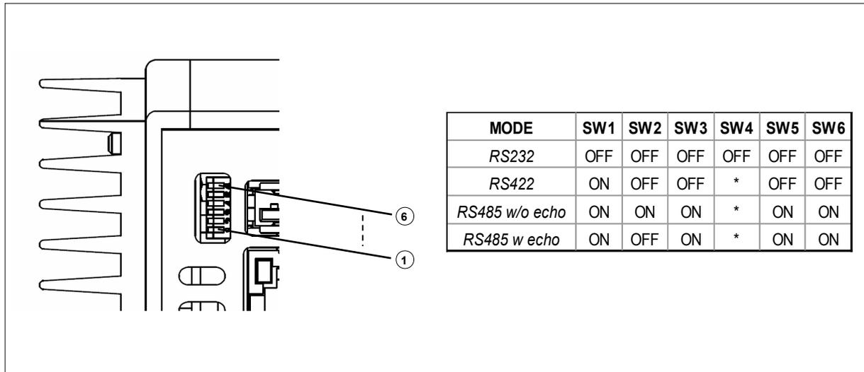
\* = This switch activate (ON) or deactivate (OFF) the resistor termination of receiver line; set it as application needs.
